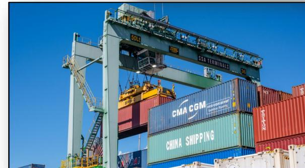
**ZE grid-electric rubber-tired gantry crane**
