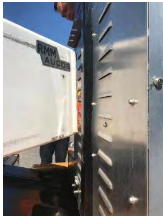
Figure 33: The fuel tank with clear impact markings from the 5 th wheel
