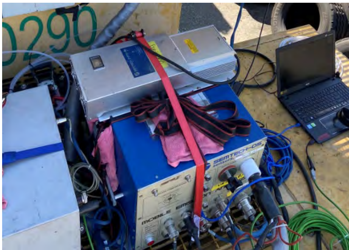
Figure 5. Picture of Semtech DS PEMS installed on the top handler.
