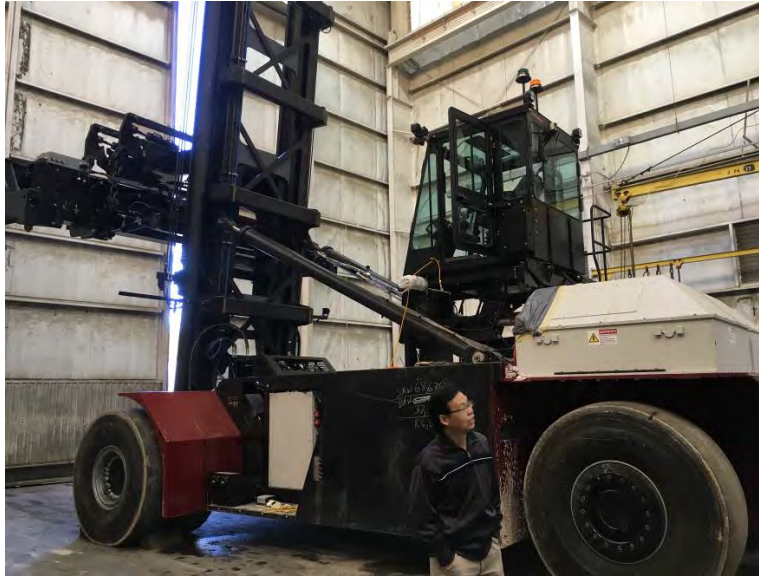
Figure 3: Operational Stage (includes fully assembled truck with mast and spreader. Unit is fully assembled and being prepared for testing)
