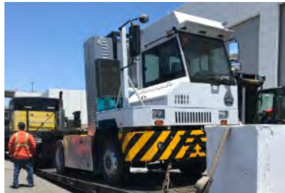
Figure 3: Kalmar and TransPower/Meritor battery electric yard tractor at LBCT (left), and CNHTC/Sinotruck and Loop Energy fuel-cell yard tractor at LBCT (ultimately removed from the demonstration) (right)
