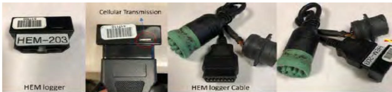
Figure 3. HEM data logger utilized for the activity monitoring program
