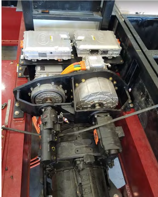
Figure 2: Electric Drive System (includes implement drive motor, steering drive motor, and related motor inverters)
