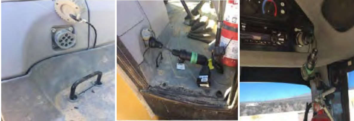
Figure 37: Outlet and HEM data logger used for the activity monitoring program
