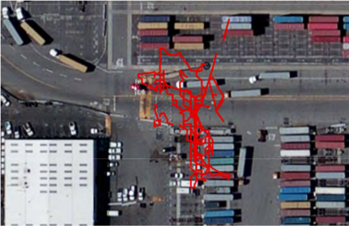
Figure 27. Data showing the routes taken over the course of a representative day for top handler #1 at the SSA Terminal on 9/21/20.
