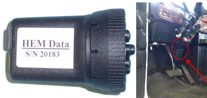
Figure 5. HEM data logger utilized for the J1939 activity monitoring program
