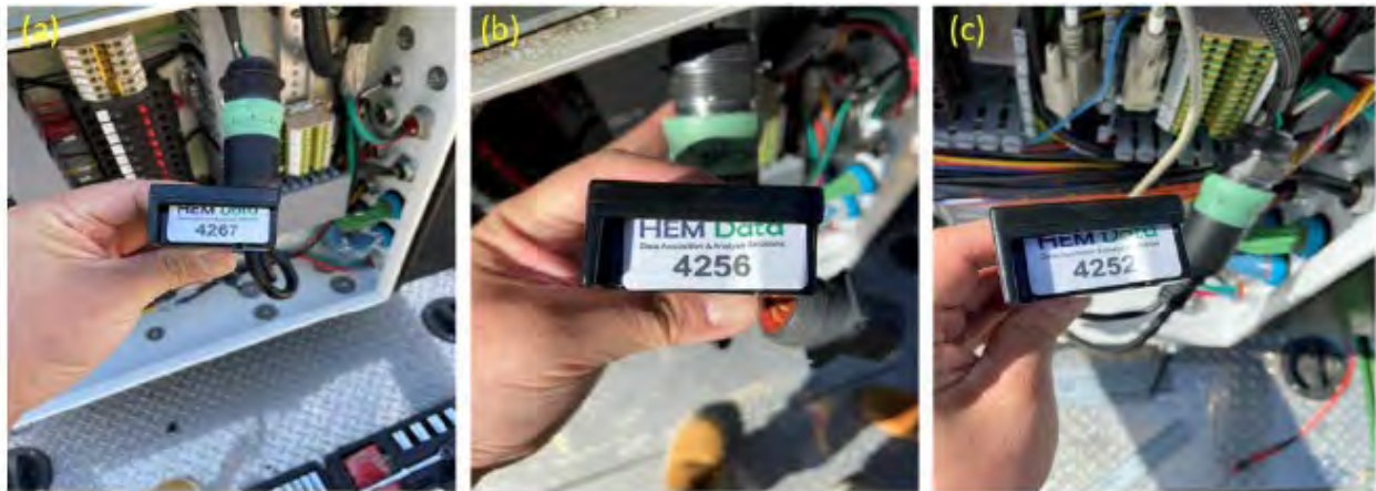
Figure 4. HEM data logger installation for a Top Handler
