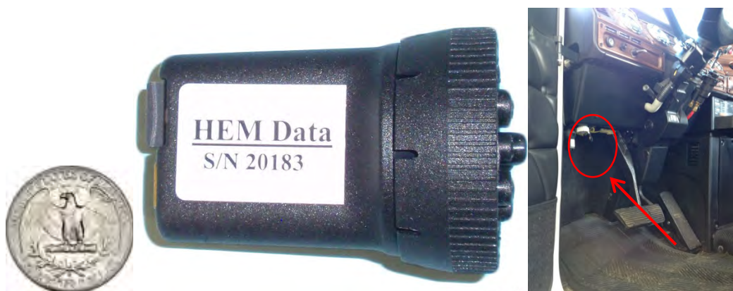
Figure 4. HEM data logger utilized for the J1939 activity monitoring program
