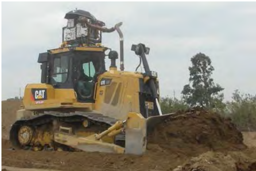
Figure 6. Picture of PEMS Rack Mounted to Construction Bulldozer
