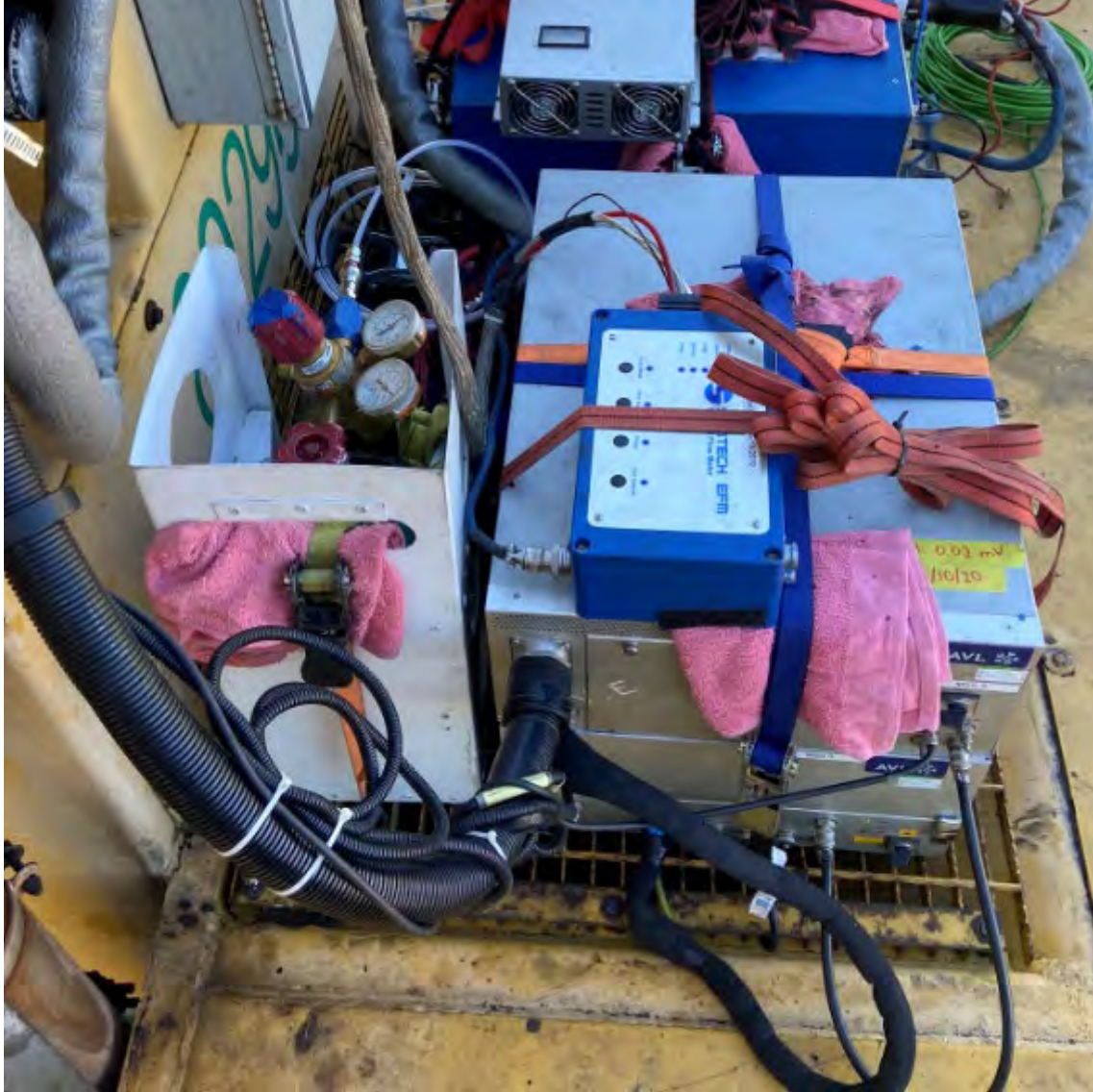
Figure 6. Picture of PM PEMS installed on the top handler.
