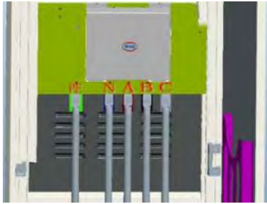
Fig. 2.14 Fixation of terminals of the cables
