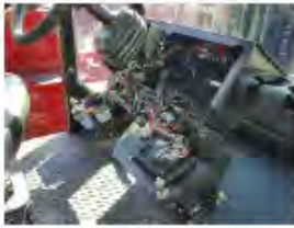
Flip-down Dash with Color/Number Coded Wiring (Standard)
