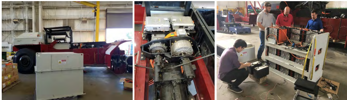
Figure 22: Partially assembled chassis and fully assembled battery pack (left), the electric drive system (center), and battery pack analysis testing with a partially assembled battery pack (right)
