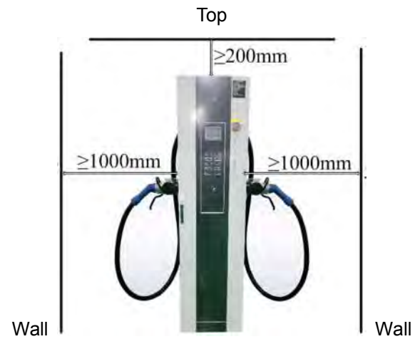
Fig. 2.1 Diagram of minimum installing distance
