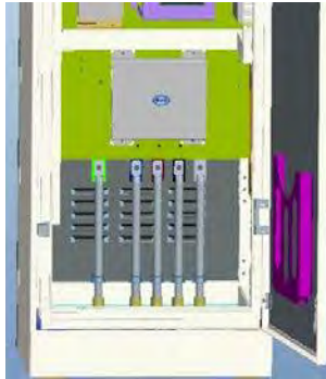
Fig. 2.11 Penetration cables into the rear closure plate
