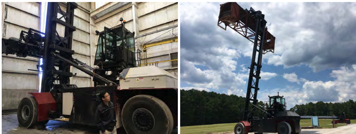
Figure 23: Operational stage buildout ready to begin testing (left) and testing and safety audit with test loads (right)
