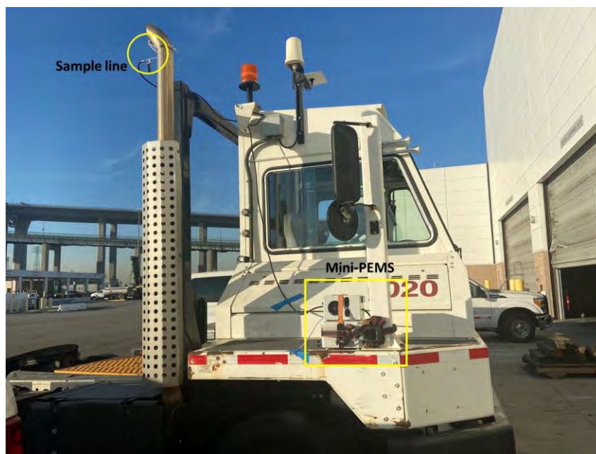
Figure 7. Picture of the mini-PEMS mounted on the Yard Tractor
