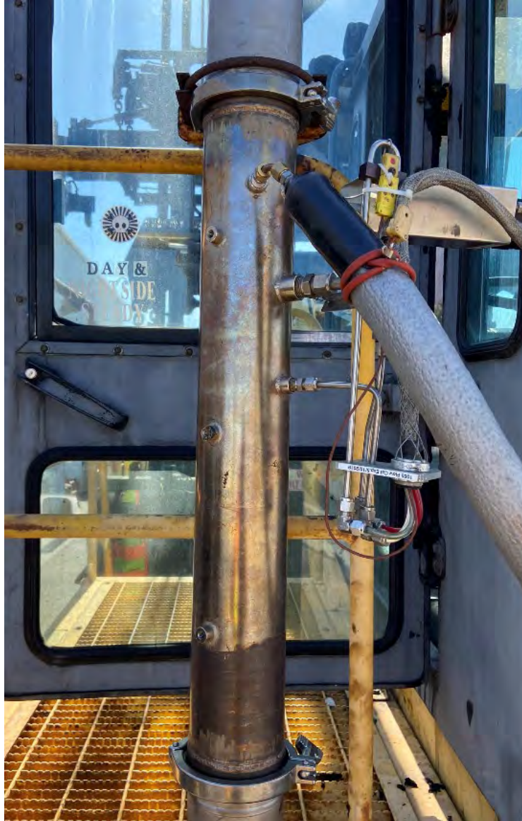
Figure 7. Picture of Sensors Exhaust Flow Meter attached to the exhaust of the top handler.
