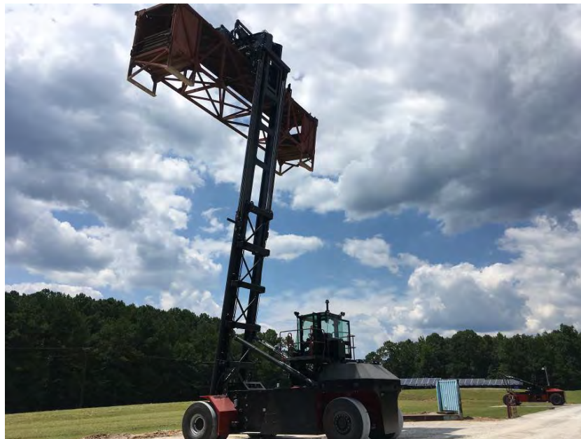
Figure 4: Testing and Safety Audit (includes operating unit, fully lifted and fully loaded using test loads. Unit located and operating at the Load Test Facility)
