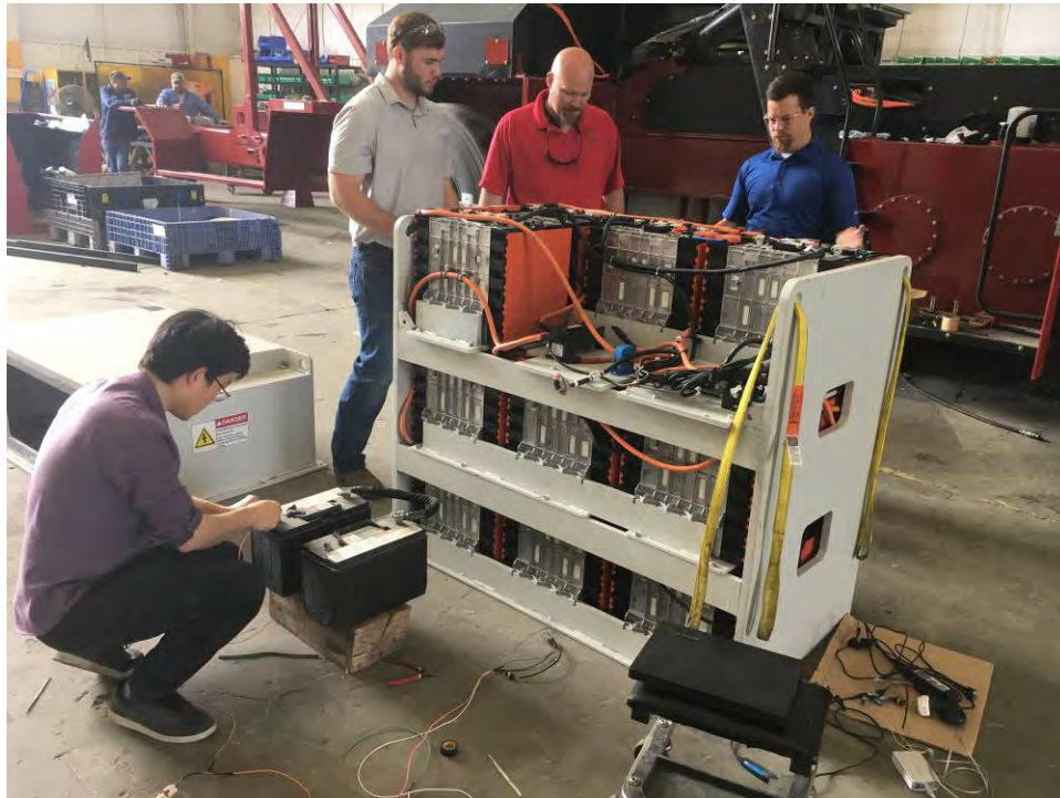
Figure 5: Battery pack analysis (includes a partially assemble battery pack including batter modules and battery pack system hardware)
