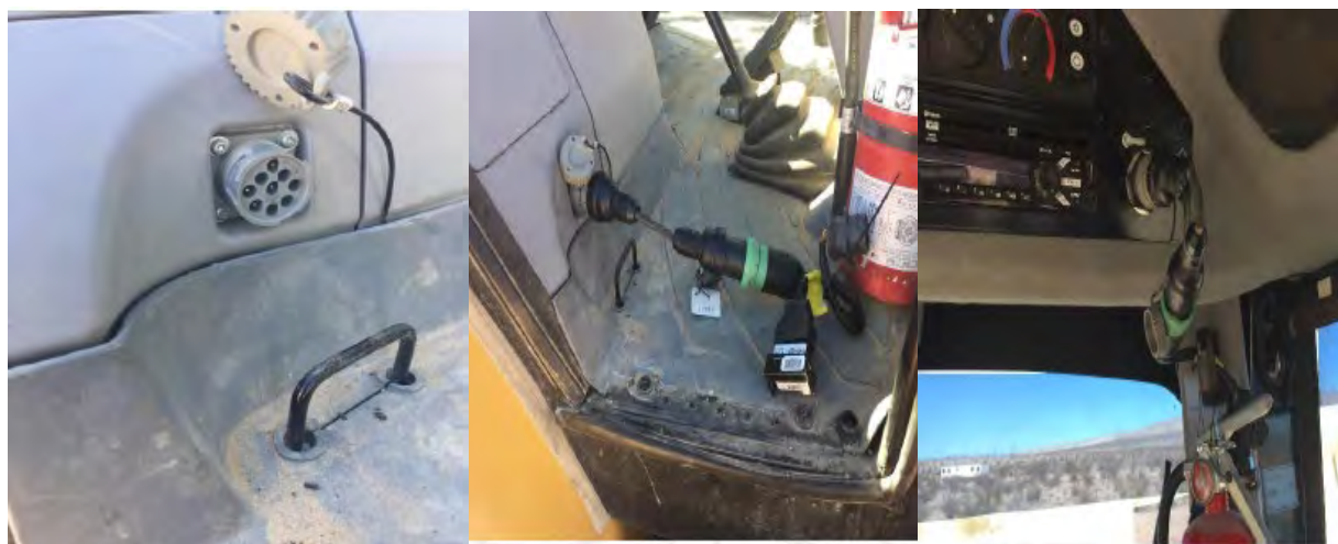
Figure 1. Outlet and HEM data logger to be utilized for the activity monitoring program
