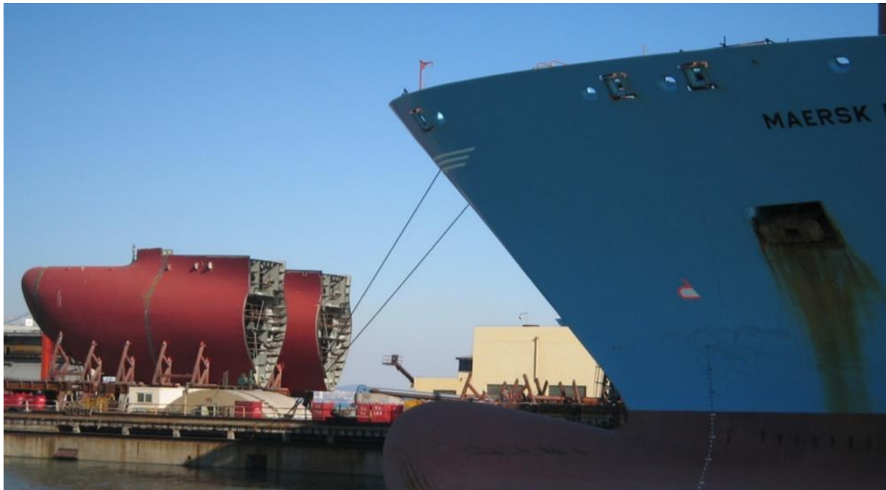
Figure 1.3: New Bulbous Bows Waiting for Installation at Shipyard
