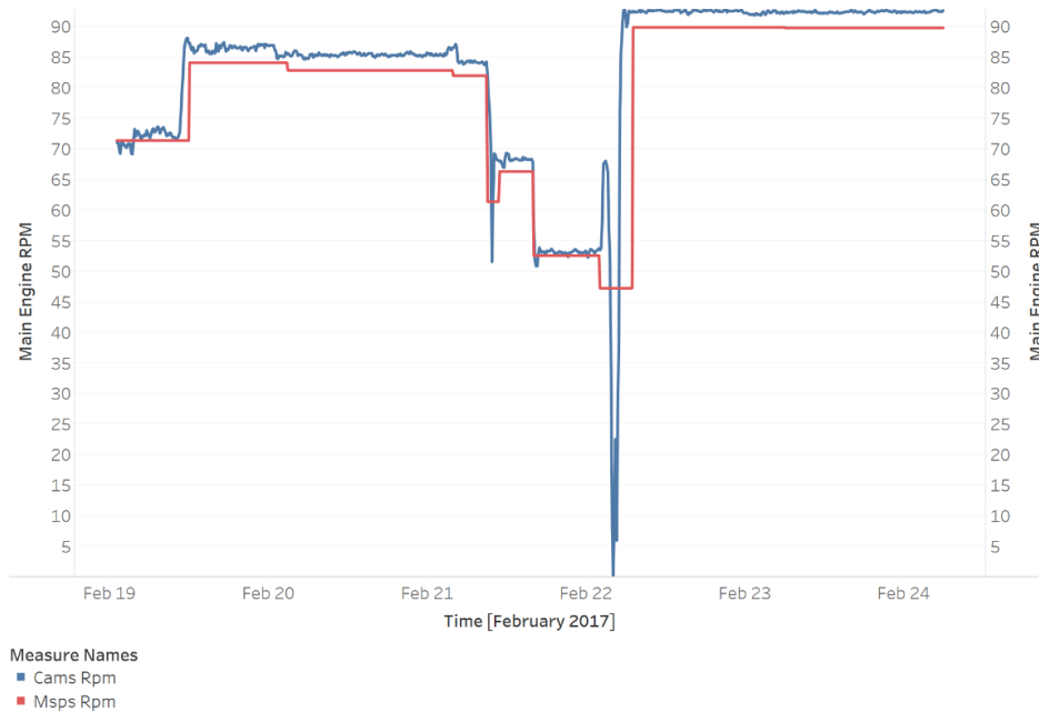
Figure 4.2: Guthorm Maersk MSPS and CAMS main engine RPM from consecutive constant ME load/normal cruising reports (Feb 19 to Feb 24, 2017). Vessel departed Singapore on Feb 18, 2017 and arrived at Suez Canal on Mar 1, 2017.
