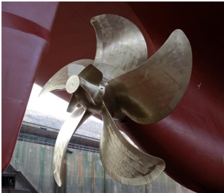
Figure 1.5: New Efficient Propeller with Boss End Caps
