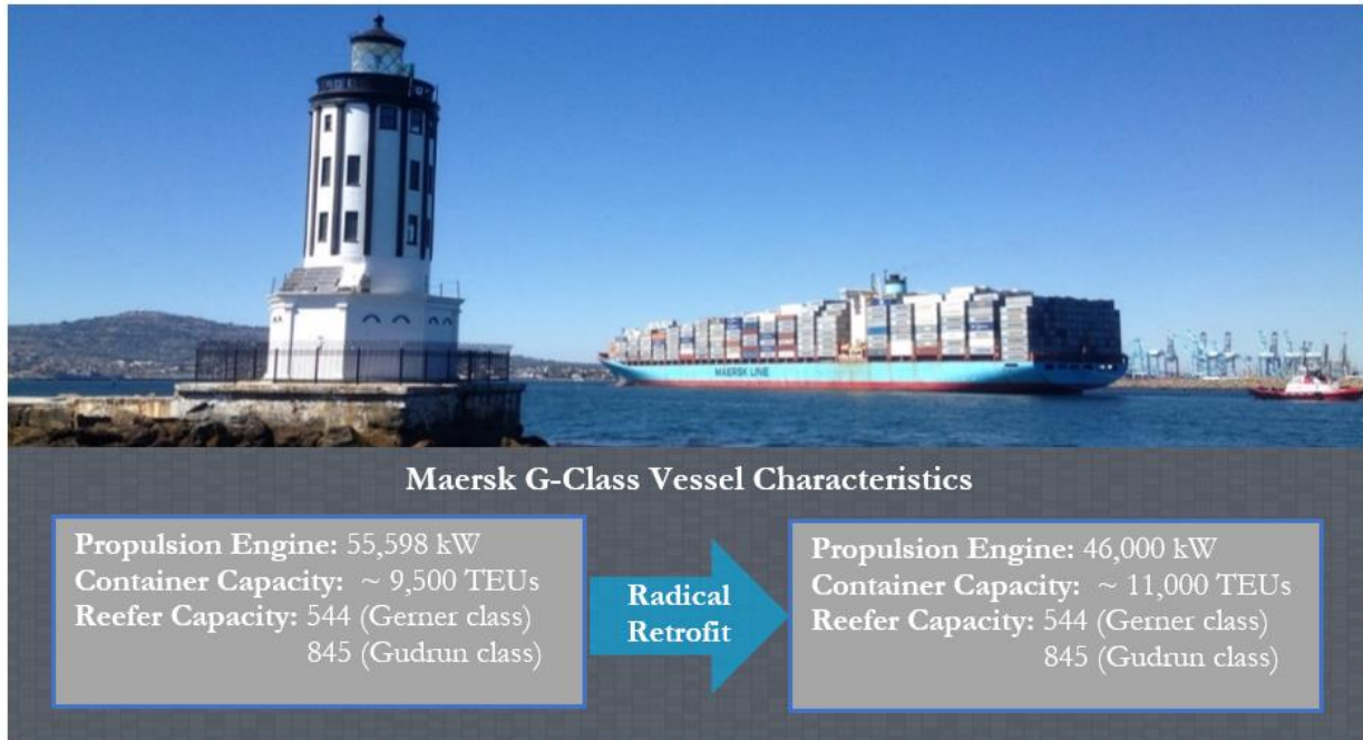
Figure 1.7: Summary Comparison of Key Parameters Pre- & Post-Radical Retrofit
