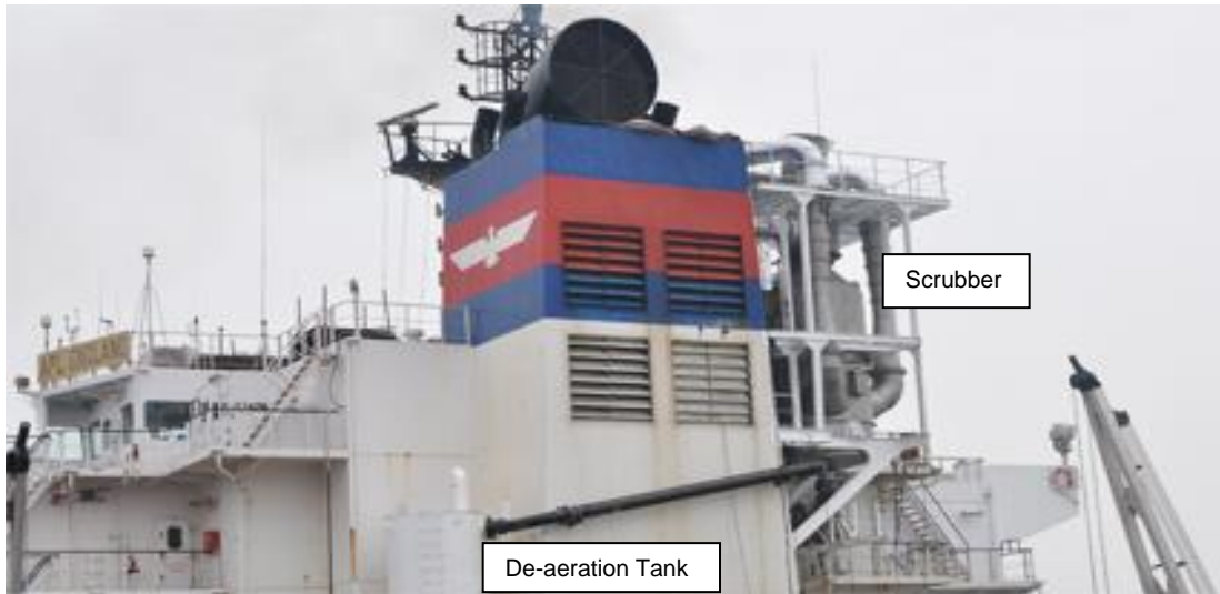
Figure 1-3: On the day of commissioning with two B&W 7L32/40's running the scrubber exhaust is clear and has no plume
