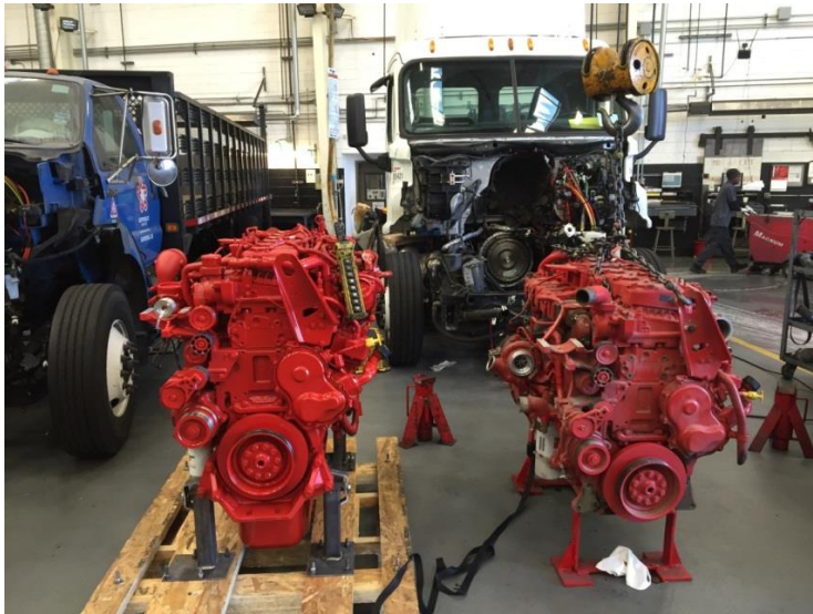
(Install process of the new, low NOx 12 Liter Engine – on left)
