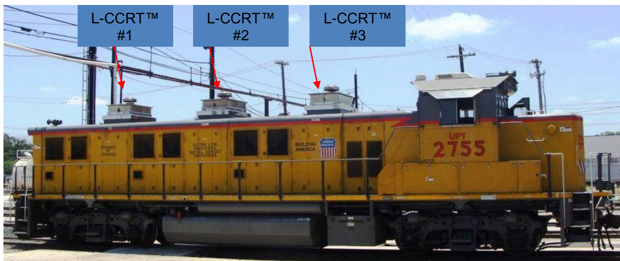
Figure 4: Union Pacific Switch Locomotive UPY-2755 fully equipped with 3 L-CCRT's
