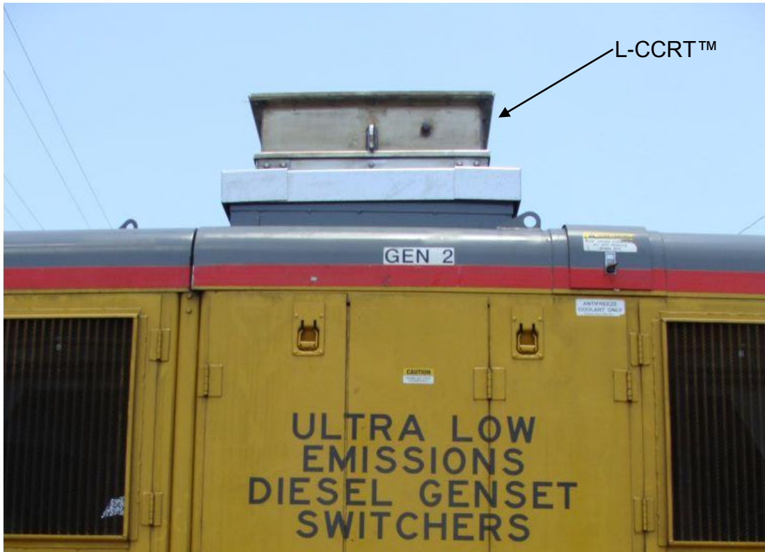
Figure 7: L-CCRT™ Installed on one genset of UPY-2755, Genset #2
