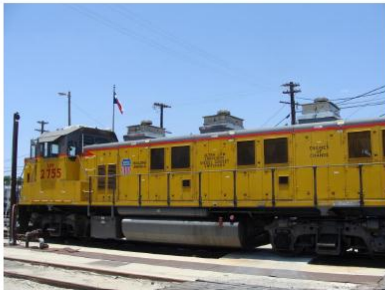
Figure 5. JM L-CCRT DPF Housings Installed
