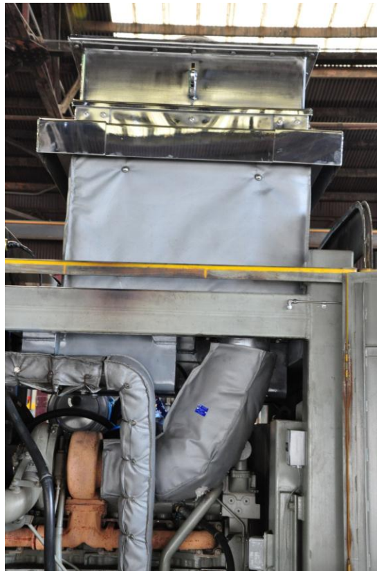
Figure 6: L-CCRT Installed on one Genset of UPY-2755, with Engine Exposed
