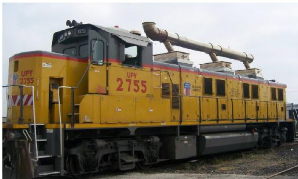
Figure 2. UPY2755 With Manifold For Collecting Exhaust From All Three Stacks
