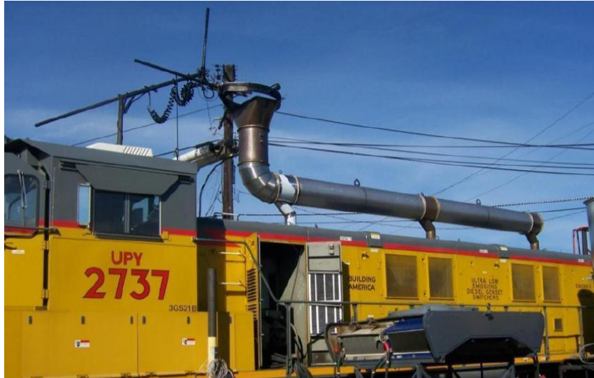
Figure 8: UPY2737 Setup for Baseline Testing by Combining All Three Exhaust Stacks
