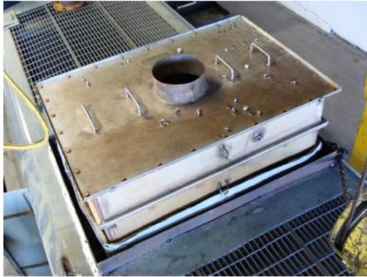
Figure 4. JM L-CCRT DPF Housing with Modified Roof Section
