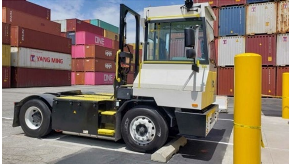
Figure 1: Two Commissioned WAVE Opportunity Charging Pads and a BYD Battery-Electric Yard Tractor
