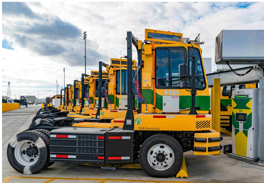
Figure 13: Zero-Emission Yard Tractors and Chargers at Port of Long Beach
