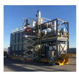
Figure 7: ShoreKat At-Berth Emissions Control System
