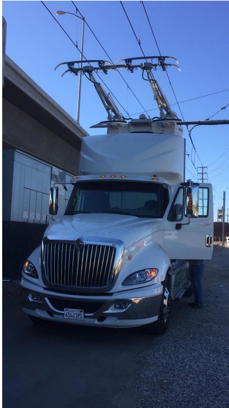
Figure 3.1: TransPower's Overhead Catenary Demonstration Vehicle
