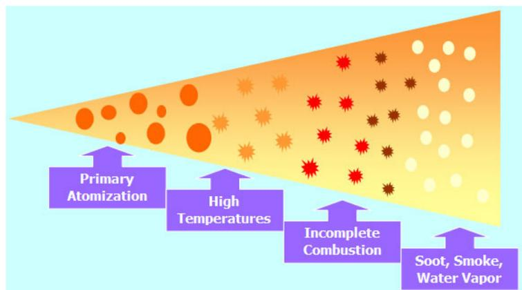
Since only the surface of each fuel droplet exposed to air can burn, larger liquid fuel droplets do not burn completely, leaving unburned carbon to collect on the surfaces of a combustion chamber or escape as PM in exhaust gases. This reduces overall thermal efficiency and increases harmful emissions, as denoted in Figure 2.2-2.
