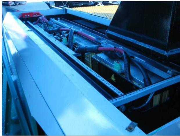
Under this follow-on TAP demonstration, one electric drayage vehicle and electric yard tractor were converted from lead acid battery to lithium battery technology. The vehicles demonstrated include:
