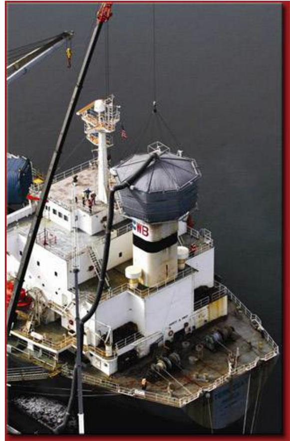
A seal closes the open area between the perimeters of the bonnet and ship's stack to limit the amount of air entering the bonnet as well as to prevent exhaust gases from escaping. The exhaust gases from the ship's auxiliary engines and the boilers are routed through a flexible duct to an Emission Treatment System (ETS) located on the dock adjacent to the vessel's berth. The ETS uses multiple exhaust gas treatment technologies to remove both gaseous and particulate pollution:
