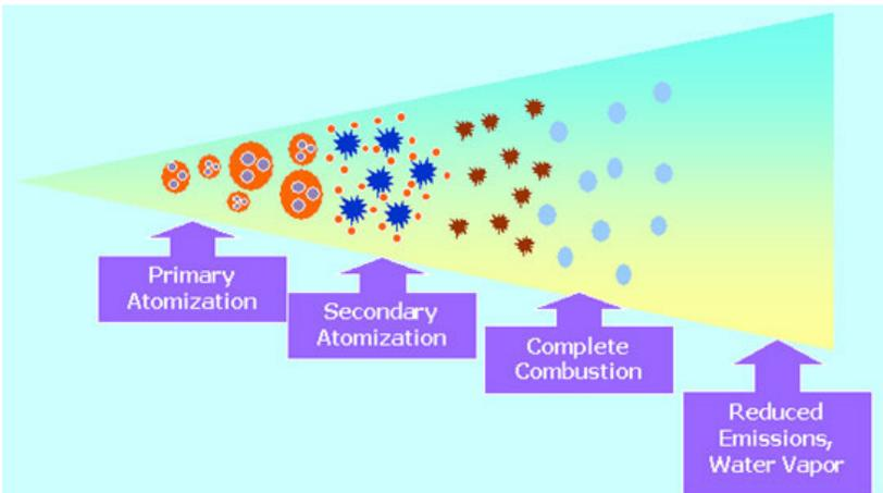
Unlike conventional diesel fuel, when emulsified fuel droplets are sprayed into the combustion chamber, they are atomized a second time as a result of the violent transformation of their water content into steam. This transformation of water into steam shatters the petroleum surrounding that water into much smaller droplets, shown in Figure 2.2-2 at left. Smaller droplets have a much
