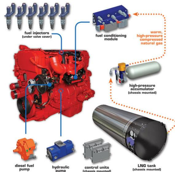
HPDI relies on late-cycle high pressure injection of natural gas into the combustion chamber. The natural gas is injected at the end of the compression stroke, similar to the diesel fuel in a diesel engine. Natural gas has a higher ignition temperature compared to diesel, so a diesel pilot injection is used to initiate combustion.
