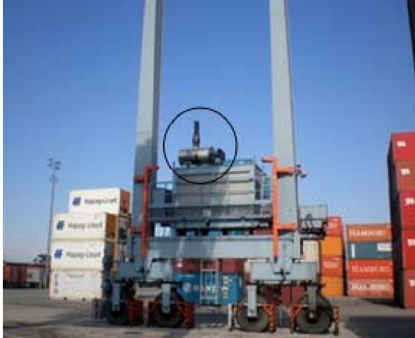
Figure 2.3: The RYPOS HDPF/C™ System Installed on an RTG Crane
