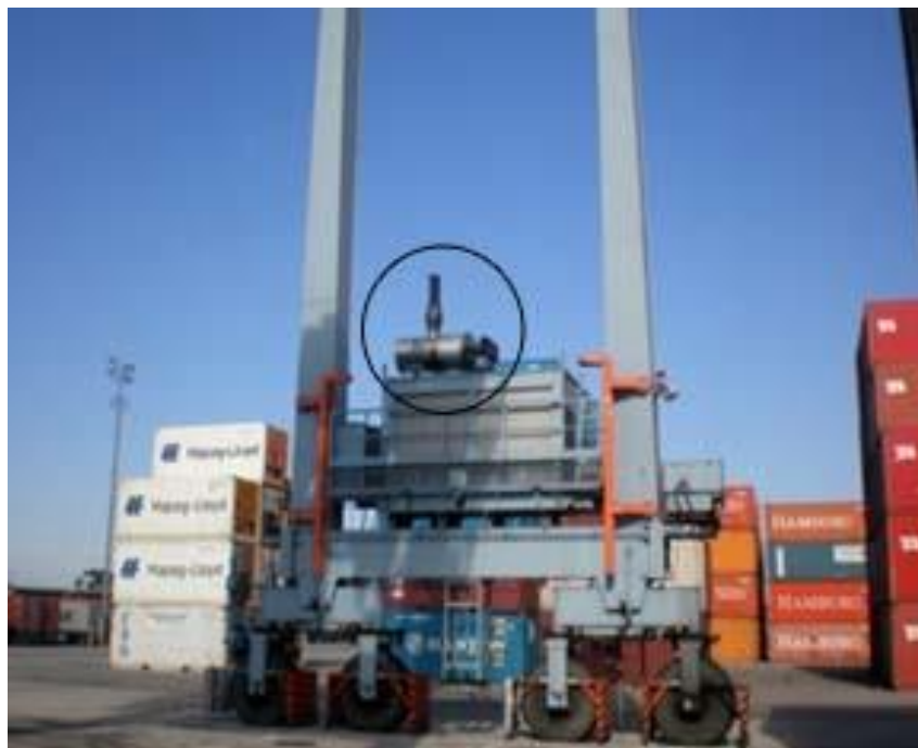
Figure 2.7: The RYPOS HDPF/C™ System Installed on an RTG Crane
