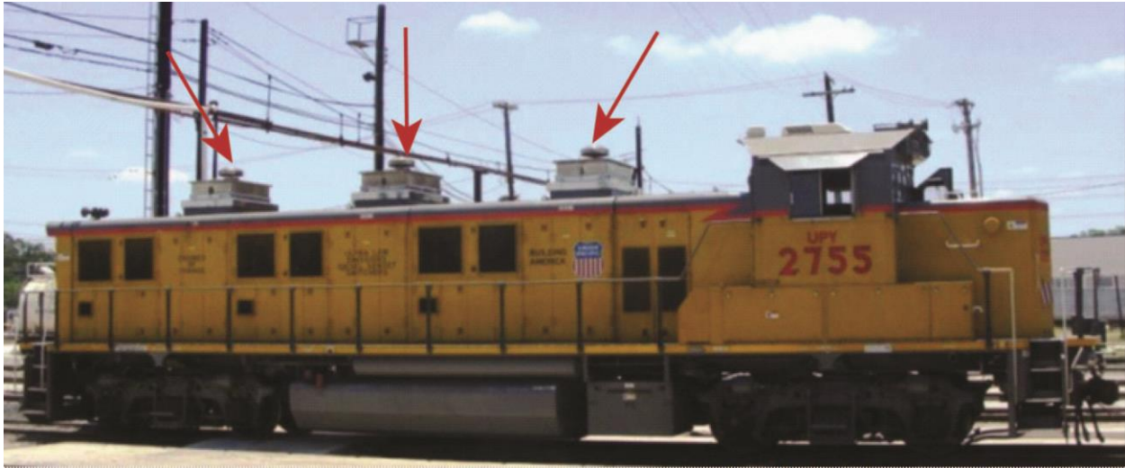
Figure 2.5: JM System Fully Installed on all three Gensets of UP2755
