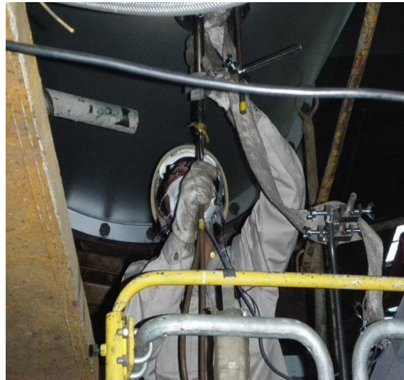
Figure 2.2: Gaseous Emissions Testing –Probe Inserted into Exhaust Duct Test Port
