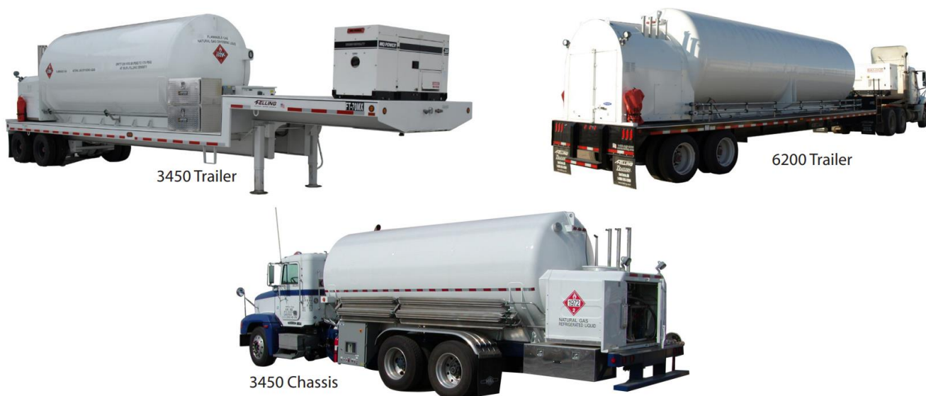
Figure 14. Examples of mobile LNG fueling stations (photos from Chart Industries)
